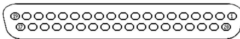
Figure 18. RCONSCSI-N-D37-1 Connector – View Facing Connector
