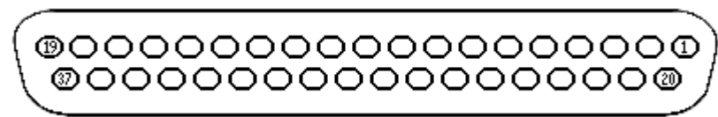
Figure 35. RAR-MPCIE Adapter Cable P1 Connector – View Facing
